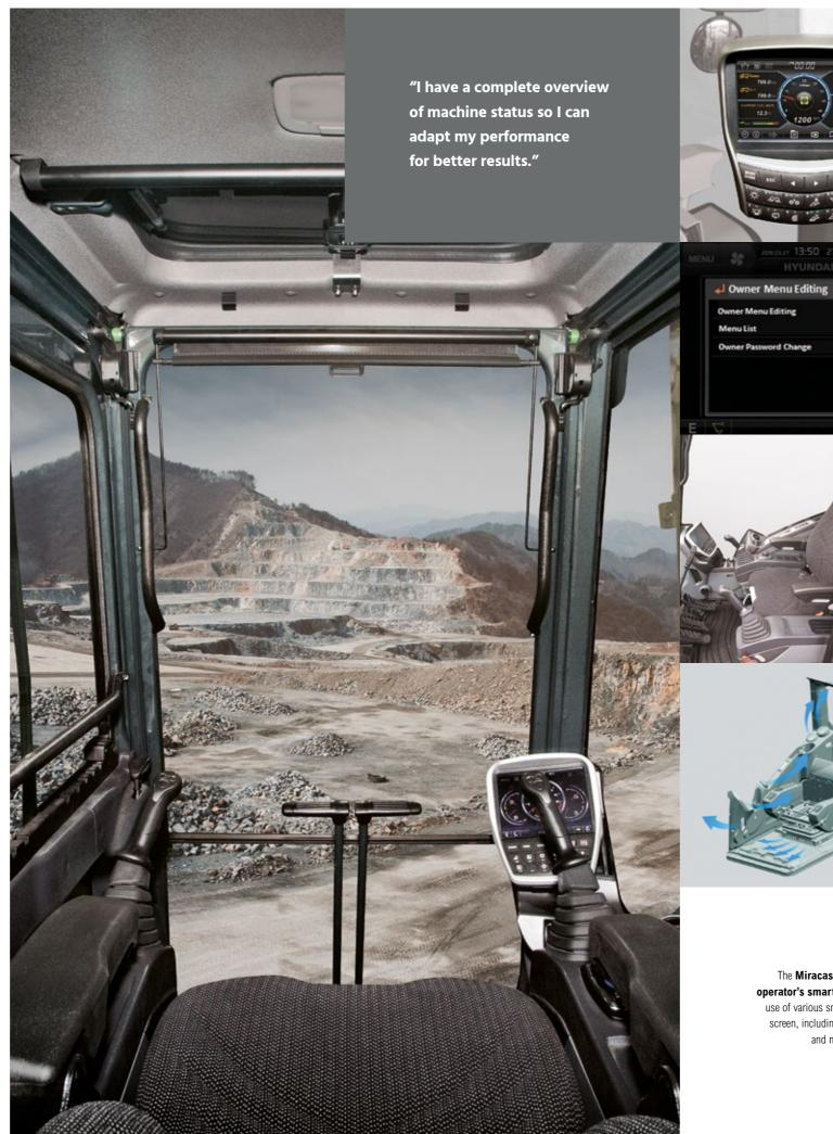
The **instrument panel** is optimised to provide quick, easy access to machine status information as you work. It features an 8-inch **touchscreen monitor** for excellent legibility.
