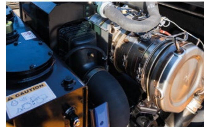
Like all A-Series machines, the HL 970A features our all-in-one exhaust aftertreatment system which cuts emissions and operating costs while enhancing reliability and simplifying maintenance.
