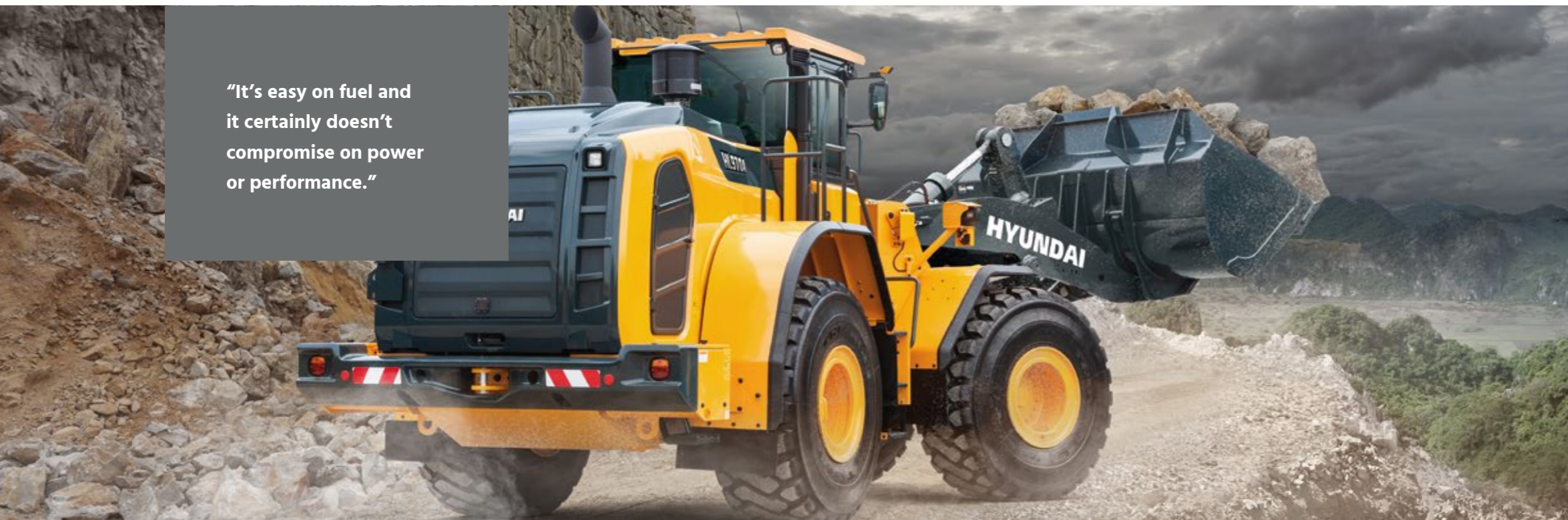
The new Smart Power mode adjusts engine RPM in heavy load work like digging to save fuel without compromising on performance. The technology also achieves an optimal balance between traction and breakout forces.
