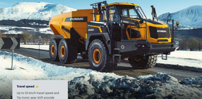
Up to 55 km/h travel speed and Tip-tronic gear shift provide smoother operation whilst maintaining maximum momentum. The truck can also be run in both automatic and manual gears.
